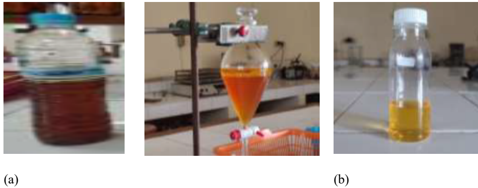
Figure 2. (a) The used cooking oil, (b) biodiesel product separation process, and (c) biodiesel product
