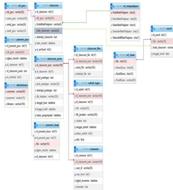
Figure 10. Entity Relationship Diagram
